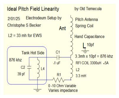
R1-10 ohm Potentiometer in series with the RF choke and ground can sweep the full audio pitch range. This Pot verifies if the Electrodeum circuit is resonating which validates *"ideal pitch field linearity"* is **On**.
