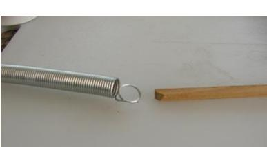
Shove the ¼" wood stick all the way to the opposing spring end, then mark where shown below. Add ½" to the right, cut the stick and insert it in behind the cross loop for a ½" stretch on the spring. Epoxy spring to the stick on each end.
