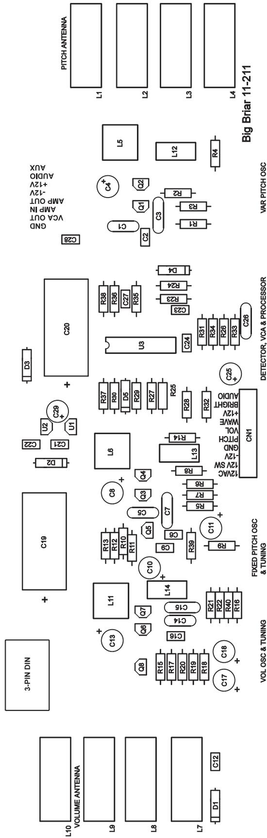
Figure 4 - Component Layout of Etherwave Circuit Board
