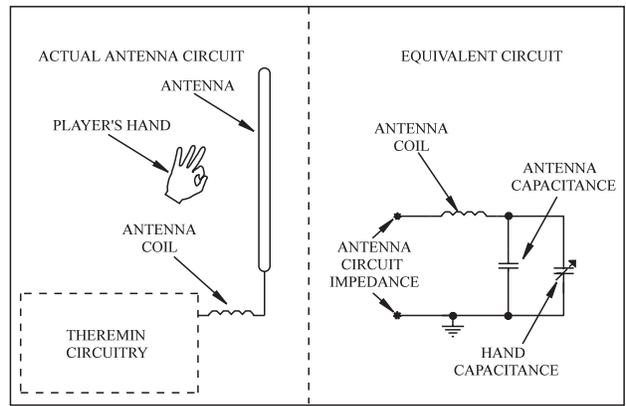
Figure 1 - Equivalent Circuit of Hand Capacitance
