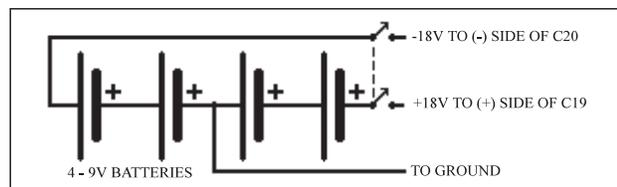
ground. A double-pole switch may be used to turn on the batteries. Figure 5 shows how to hook four 9-volt batteries to power your *Etherwave* in the absence of regular AC power. Keep in mind that the *Etherwave* draws about 30 milliamperes, so a set of four regular 9-volt batteries will last for only a few hours.
